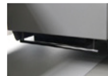
Anti-collision device prevents PH damage during printing
