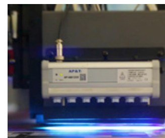
Anti-collision device prevents PH damage during printing
