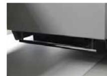
Anti-collision device prevents PH damage during printing
